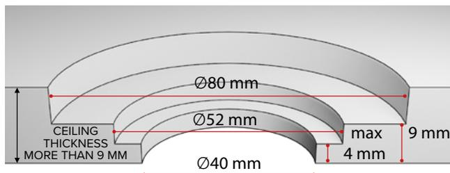
EN: Cut a hole from the back side of the panel with a diameter of 40 mm / 1,57". Cut a hole with a diameter of 80 mm / 3,15" until you reach a ceiling thickness of 9 mm / 0,35". Cut another hole with a diameter of 52 mm / 2,1". Leave max 4 mm / 0,16" of the ceiling intact. Remove any burr.
