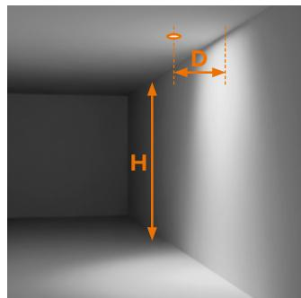
The **spacing between luminaires (S)** shall be minimum the distance (D) from the wall and maximum twice the distance (D x 2) from the wall
