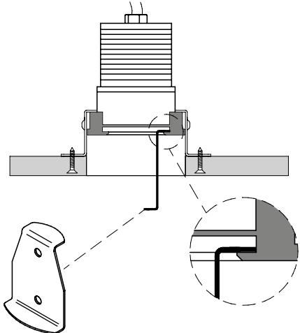
2 EN: Pull the key downwards to unlock the luminaire.
