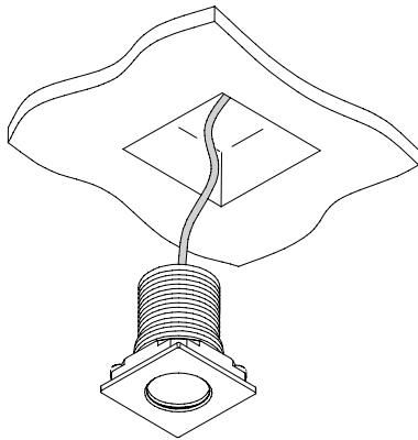
**2** EN: Push the luminaire up to the end and be careful not ruining the inner walls of the mounting frame. The magnets will hold it in place.
