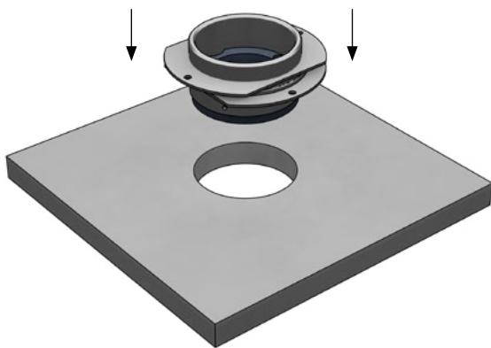
**3** Remove the upper bezel from the housing box and insert it into the hole.
