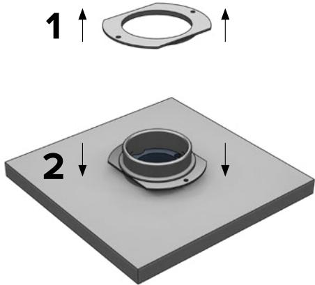
**4** Make sure the plastic spacer is flush with the ceiling and fix the mounting frame with screws.
