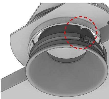
**9** EN: Pushing the luminaire towards the mounting frame, rotate it clockwise until it stops.
