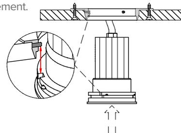
EN: Proper heat dissipation is required when installing the luminaire and, therefore, provide an empty area in the back of the luminaire. Do not sink the luminaire within any materials with low thermal conductivity such as wood, plastic, etc. and do not fix the luminaire with resin, polyurethane foam or silicon.
