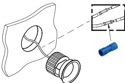
2 EN: Insert the luminaire in the mounting frame, paying attention that the three luminaire's slots match the three mounting frame's pivots.
