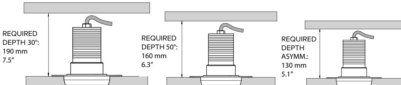
**2** EN: Make a hole in the wood panel and remove any burr.
