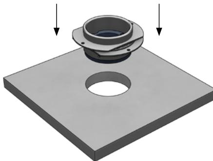
**4** EN: Remove the upper bezel from the mounting frame and insert it into the hole.
