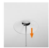
MAINTENANCE SYMMETRICAL Remove luminaire by pulling the hex key
