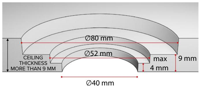
Cut a hole from the back side of the panel with a diameter of 40 mm. Cut a hole with a diameter of 80 mm until you reach a ceiling thickness of 9 mm. Cut another hole with a diameter of 52 mm. Leave max 4 mm of the ceiling intact. Remove any burr.
