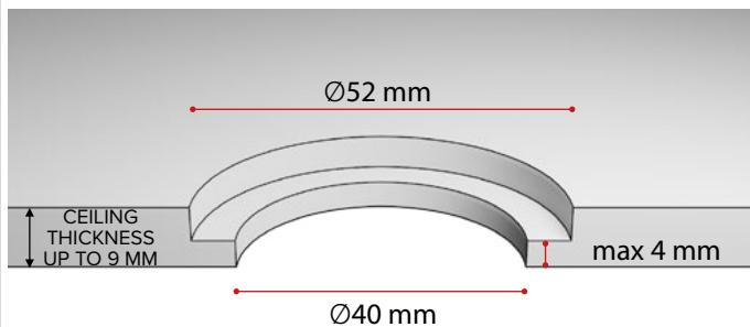
Cut a hole from the back side of the panel with a diameter of 40 mm. Cut another hole with a diameter of 52 mm. Leave max 4 mm of the ceiling intact. Remove any burr.
