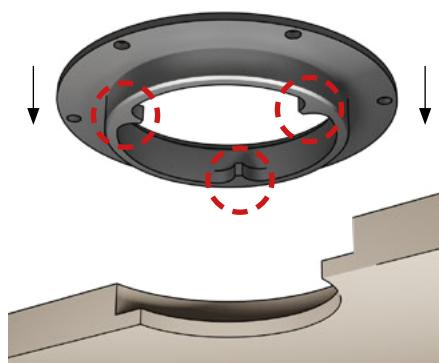
**3** Adjust the ring and fasten with the included screws.
