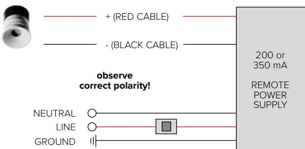
**WIRING EXAMPLE DALI OR 1-10V: 200 or 350 mA**
