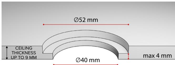
EN: Cut a hole from the back side of the panel with a diameter of 40 mm / 1,57". Cut another hole with a diameter of 52 mm / 2,1". Leave max 4 mm / 0,16" of the ceiling intact. Remove any burr.
