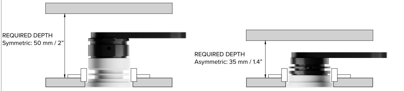
**2a** EN: Ceiling thickness up to 9 mm / 0,35".
