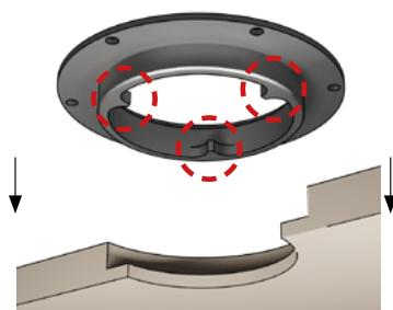
**4** EN: Adjust the ring and fasten with the included screws.
