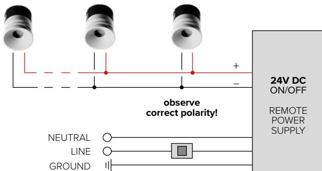
**WIRING EXAMPLE DALI OR 1-10V: 24V DC**
