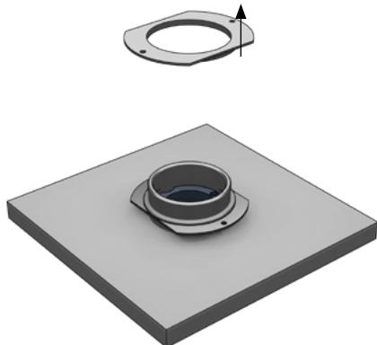
**5** EN: Make sure the plastic spacer is flush with the ceiling and fix the mounting frame with screws.
