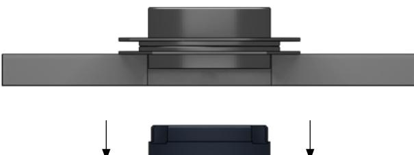
**8** EN: Insert the luminaire in the mounting frame, paying attention that the three luminaire's slots match the three housing box's pivots.
