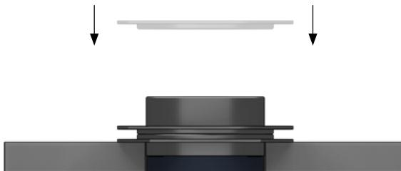
**7** EN: Remove the plastic spacer.
