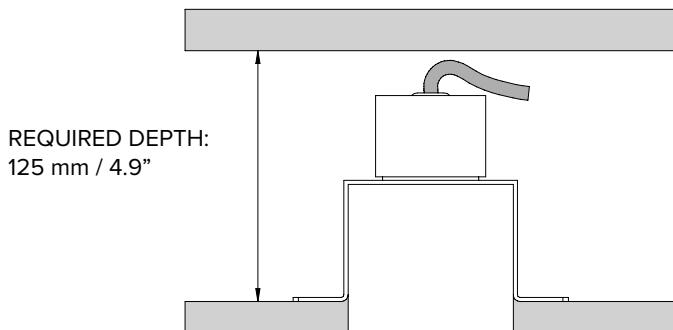
**2** EN: Place the mounting frame on the plasterboard and draw a hole.
