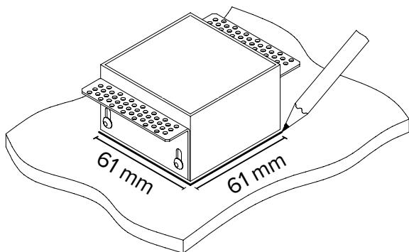
**3** EN: Make a hole in the plasterboard.
