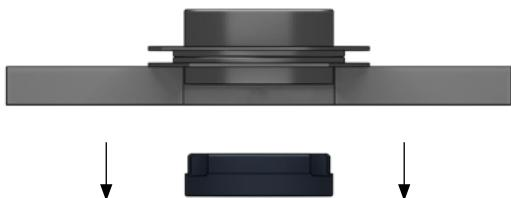
**8** EN: Insert the luminaire in the mounting frame, paying attention that the three luminaire's slots match the three housing box's pivots.
