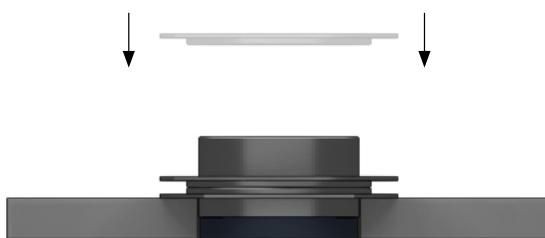
**7** EN: Remove the plastic spacer.
