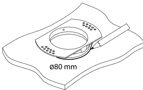
3 EN: Make a hole in the plasterboard.
