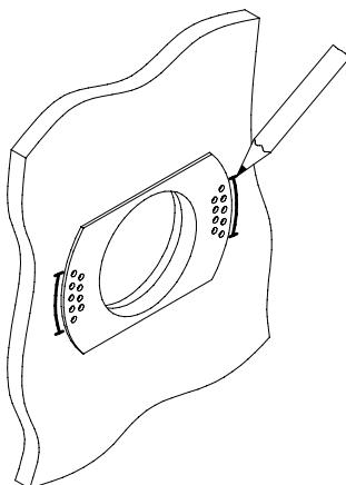
5 EN: Insert the mounting frame by tilting it.
