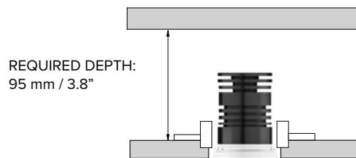
**2** EN: Make a hole in the wood panel and remove any burr.
