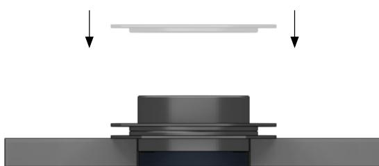
**7** EN: Remove the plastic spacer.
