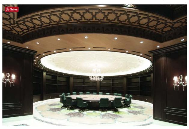
General and accent lighting are provided by a bespoke system of 140 gimbals, created following the designer's specifications, each adjusting five projectors and managed by a sophisticated DXM control. The selected light sources for this project were high emission LED lamp sources with a color temperature of 3000K and CRI93.
